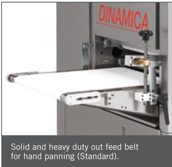
Solid and heavy duty out feed belt for hand panning (Standard).
