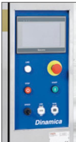
The panel also has a diagnostics screen to identify possible operational problems. Further, the panel can identify conflicts where the dough weight, the production speed, and, the overall machine speed are non-synchronous, mechanically or through the potentiometer.
