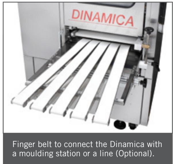
Finger belt to connect the Dinamica with a moulding station or a line (Optional).
